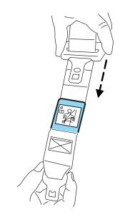
4. Store the belt in the housing found on the ceiling by inserting the smaller tongue in the slot provided.
